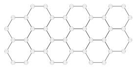
This is a single plane of graphite, called *graphene*. A piece of graphite consists of many of these planes, layered. The chemical bonds between the planes are much weaker than the bonds inside the planes, which explains why pencils write—the graphite can be sheared so that the planes slide off and are left on the paper.
