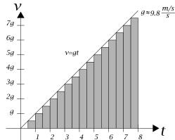
Estimate of distance traveled for  $t = 8 \& \Delta t = .5$ , using the velocity at the beginning of each interval.
