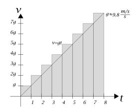
Estimate of distance traveled for  $t = 8 \& \Delta t = 1$ , using the velocity at the end of each interval.
