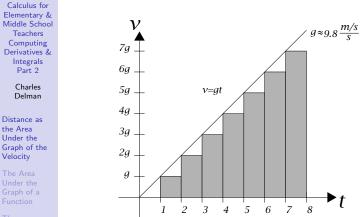
Estimate of distance traveled for  $t = 8 \& \Delta t = 1$ , using the velocity at the beginning of each interval.
