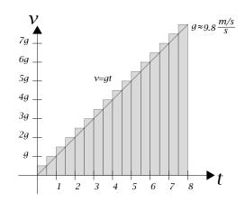
Estimate of distance traveled for  $t = 8 \& \Delta t = .5$ , using the velocity at the end of each interval.
