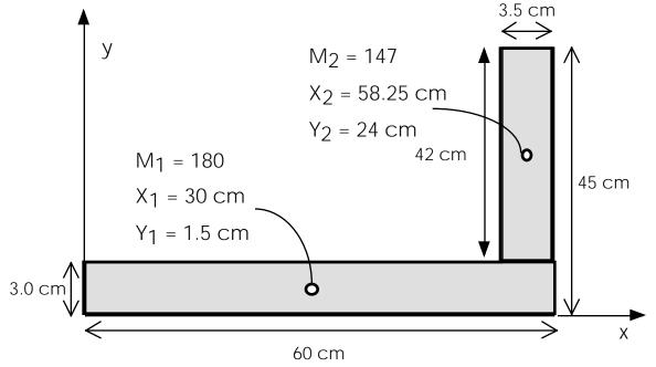
Notice that the positions are all measured from the lower left corner of the carpenter's square. Now we can use the definitions of center of gravity, Equations 8.10 and 8.11, to locate the center of gravity of the entire object,
