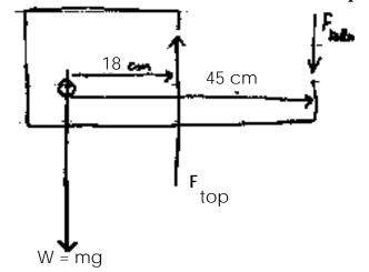
Now apply the second condition of equilibrium,  $\tau_{ccw} = (18 \text{ cm})F_{top} = (45 \text{ cm}) F_{vottom} = \tau_{cw}$   $(18 \text{ cm})F_{top} = (45 \text{ cm}) F_{vottom}$   $F_{top} = (45/18) F_{bottom}$   $F_{top} = 2.5 F_{bottom}$   $F_{top} = F_{bottom} + 100 \text{ N}$   $2.5 F_{bottom} = F_{bottom} + 100 \text{ N}$   $1.5 F_{bottom} = 100 \text{ N}$   $F_{bottom} = 66.7 \text{ N}$
