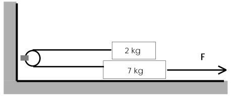
The <u>maximum</u> external force F that can be exerted will be the force exerted when the friction forces are at their maxima,
