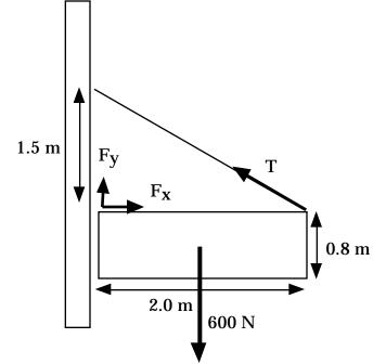
Call the components of the force exerted by the pin  $F_x$  and  $F_y$ . The angle between the guy wire and the horizontal is
