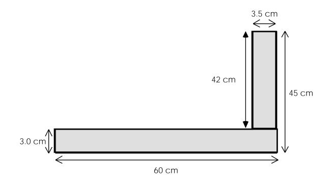
The center of gravity of <u>each</u> rectangle is at the geometric center of that rectangle and the mass (or weight) located at that position is proportional to the area of that rectangle.
